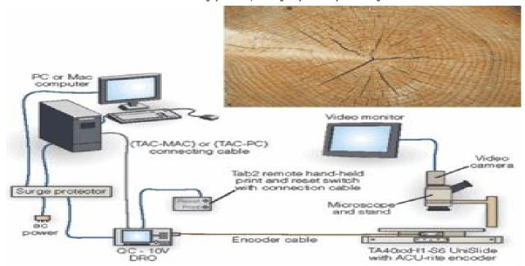
In the development of a microscopy-based positioning system for scientists studying tree-ring growth, Velmex TA system uses its own UniSlide positioning system coupled to a linear encoder and digital readout.
